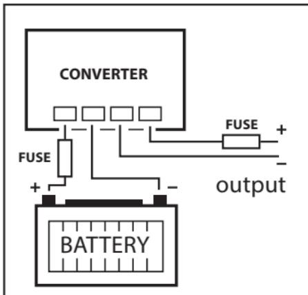
**Attention: The DC currents can be very high. Always use cables of sufficient cross sectional area (mm<sup>2</sup>)!**
