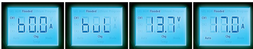
Charge Current      Charge Stage      Charge Voltage      Charger with Silent Mode On
