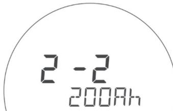
The default battery capacity value is 200Ah. This can be changed by pressing the left or right arrow keys until the desired value is reached. The standard battery capacity value is based on a discharge rate of 20 hours. When your battery capacity is rated at a different discharge rate,
