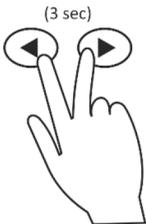
Besides automatic synchronisations, you can also manually synchronize the battery monitor, when you are sure that your battery is fully charged. This can be accomplished by pressing both left and right arrow keys simultaneously for three seconds. After these three seconds, the SoC value will be reset to 100%.
