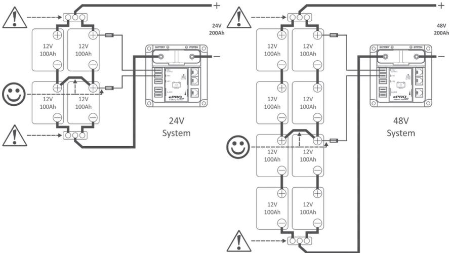
The above images are also indicating that busbars are being used to respectively join all positive and all negative battery cables. Besides this, all positive and negative battery cables that are wired to these busbars need to be of equal length. These precautions are made to avoid any imbalance between the different series strings, to ultimately improve the overall accuracy of the midpoint voltage measurement.
