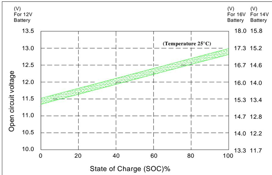
figure 2:Open Circuit Voltage Vs. State of Charge(SOC)
