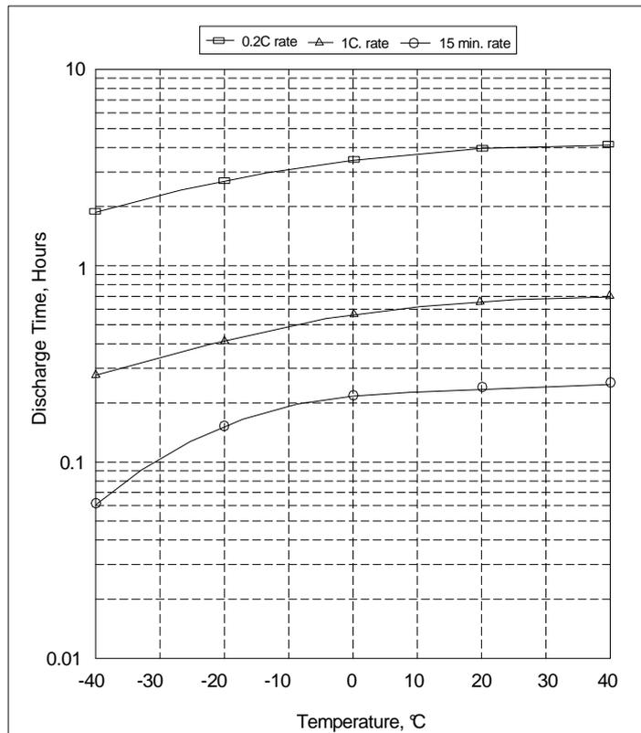
Figure 3: capacity Vs. Ambient Temperature
