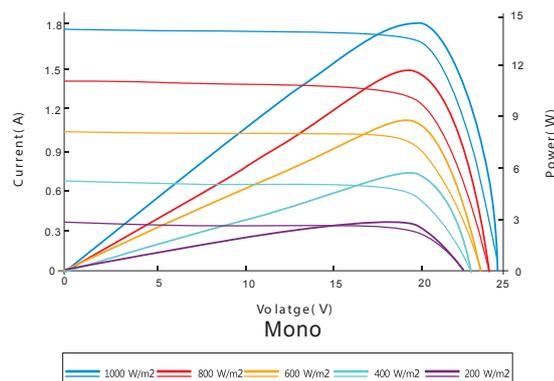
Excellent performance under weak light conditions: at an irradiance intensity of 800W/m<sup>2</sup> (AM 1.5, 25°C), 95.5% or higher of the STC efficiency(1000W/m<sup>2</sup>) is achieved.
