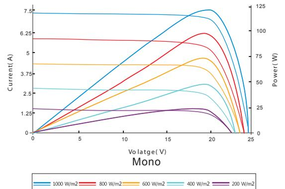
Excellent performance under weak light conditions: at an irradiance intensity of 800W/m<sup>2</sup> (AM 1.5, 25°C), 95.5% or higher of the STC efficiency(1000W/m<sup>2</sup>) is achieved.
