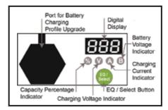
Charger will enter charging model when connecting to battery & AC input cable. Digital display on the front panel will show in turn: AC XXX (Current AC input voltage), CPU X.XX (corresponding software version number), b\*\*(Current charging profile code).
