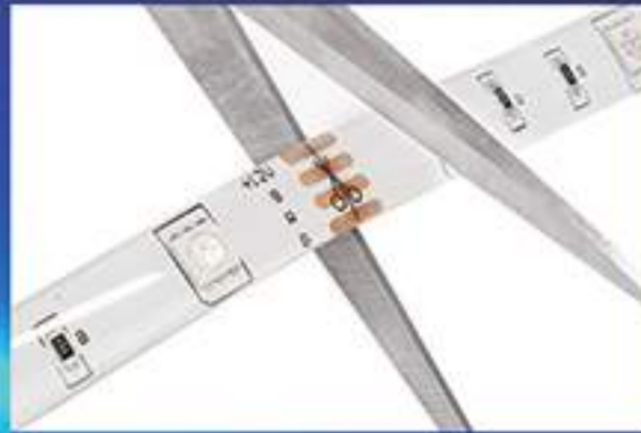
Every 3 LEDs can be cut apart
