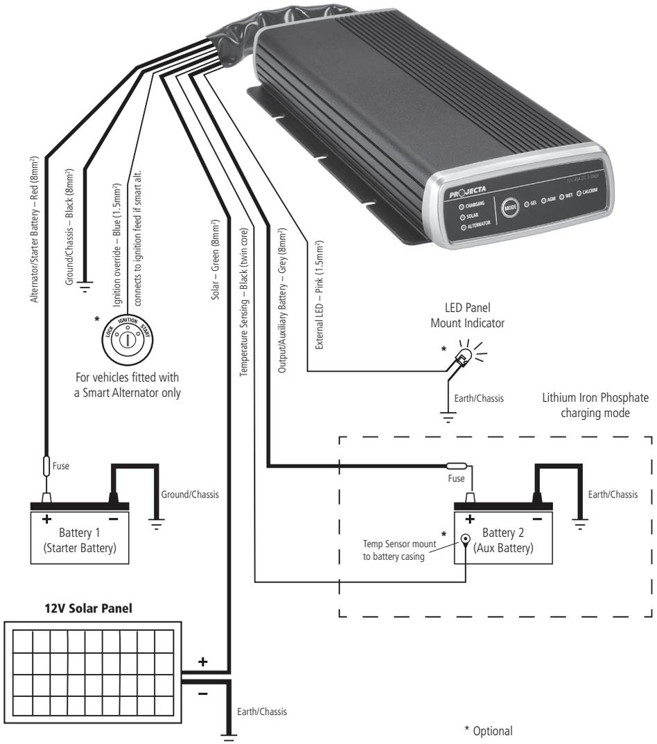
**Important:** For 24V vehicles, a battery master switch is required to connect a 12V solar panel to the IDC45 solar input. This switch is used to turn the solar panel on and off. When solar power is too low to provide fast charge to the auxiliary battery, by turning off the 12V solar panel, IDC45 can provide fast charge through alternator input.
