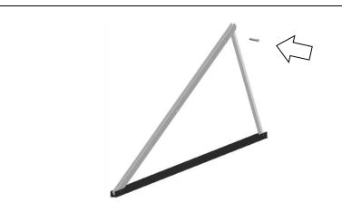
5.1.3 Fix the tubes with U Bracket to the base support by using hex head bolts M10\*65, Spring Washer, Flat Washer and Hex nuts M10.
