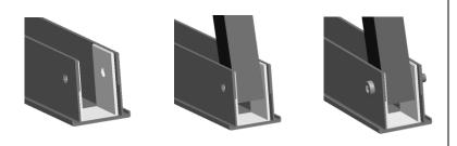
5.1.2 Unfold the middle tubes in the upper support (if you use double Tripod), fix them to the base support by using hex head bolts M10\*65 and Spring Washer, Flat Washer and Hex nuts M10.
