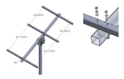
2) Preassemble the Cross Connection Clamp at the Rectangular Tube-Master with M8\*70 hex bolts, plain washer 8, spring washer 8, and M8 nut as shown in the figure below.
