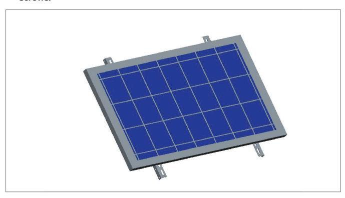
2. Fix the L feet to the brackets with M8 screws.
