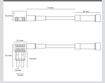
The Alvolta Micro Blade "Add A Circuit" Fuse Holder allows you to upgrade your existing fuse holder or box by adding a protected circuit. No splicing is required. Simply plug into existing fuse slots for additional circuit protection.
