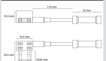
The Alvolta Mini Blade "Add A Circuit" Fuse Holder allows you to upgrade your existing fuse holder or box by adding a protected circuit. No splicing is required. Simply plug into existing fuse slots for additional circuit protection.
