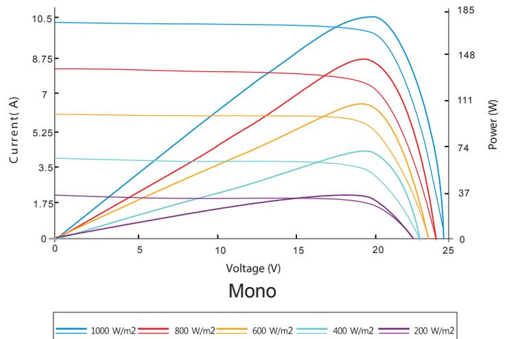
Excellent performance under weak light conditions: at an irradiation intensity of 800W/m<sup>2</sup> (AM 1.5, 25°C), 95.5% or higher of the STC efficiency(1000W/m<sup>2</sup>) is achieved.
