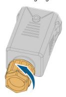
step 3 Thread the AC cable through the swivel nut, appropriate sealing and waterproof cover in sequence.
