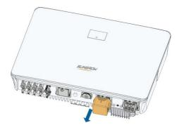
step 6 Fix all the wires to the terminals according to the assignment and tighten to a torque of 2.0 N•m with a screwdriver.
