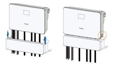
step 4 Use a screwdriver to secure screws with a torque of 1.5 N.m.
