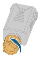
step 2 Thread the BACKUP cable through the swivel nut, appropriate sealing and waterproof cover in sequence.
