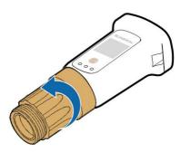
**Step 4** Thread the network cable through the swivel nut and gasket. Afterwards, route the cable into the opening of the sealing. Finally, insert the cable through the housing.
