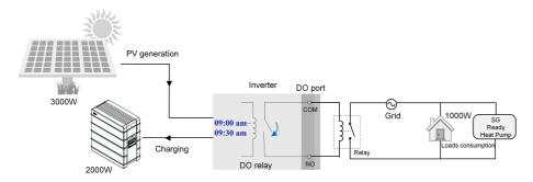
figure 8-26 DO Operation in Intelligent Mode Diagram
