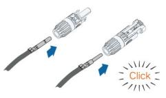
**Step 4** Tighten the cable gland and the insulator.
