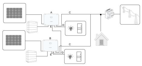
figure 2-5 Parallel PV ESS
