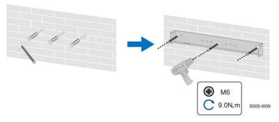
Step 3 Install the bottom bracket to avoid the inverter tilting forward.
