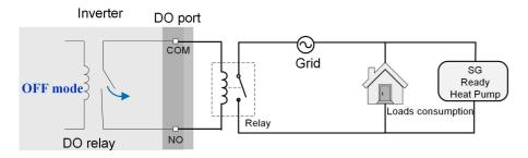
figure 8-25 DO Operation in Switch Mode Diagram
