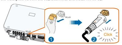
**Step 7** Slightly shake it by hand to determine whether it is installed firmly.
