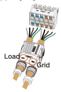
**Step 4** Strip the cable by 80 mm. If the cold-pressed terminal is to be crimped onto the cable, the cable stripping length should be 2~3 mm plus the length of the metal body of the terminal. If the cold-pressed terminal is not used, strip the cable by 14~16 mm.
