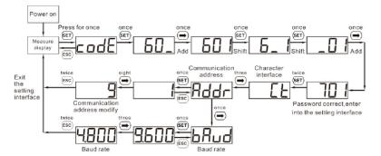
When input digits, "SET" can be used as cursor " - "motion button, "ESC" is Exit the programming operation interface or switch to the character interface from digit modification interface, add from the beginning after setting the digit to the maximum value.
