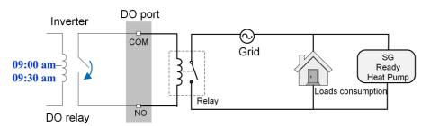
figure 8-24 DO Operation in Timing Mode Diagram
