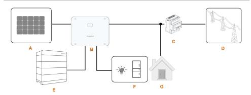
figure 2-4 PV Energy Storage System (PV ESS)
