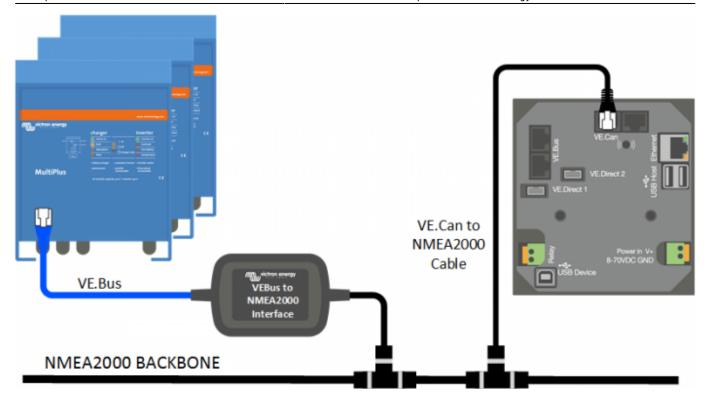
In above example, there needs to be a fuse in the VE.Can to NMEA2000 cable. Without it, the VE.Can port in the CCGX will be left without power and therefore does not work.
