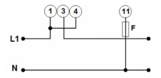
The diagram shows the wiring when used as a grid meter.
