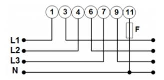
When used to measure a PV Inverter, terminals 1, 4 and 7 should face the PV inverter to ensure correct direction of current and power.
