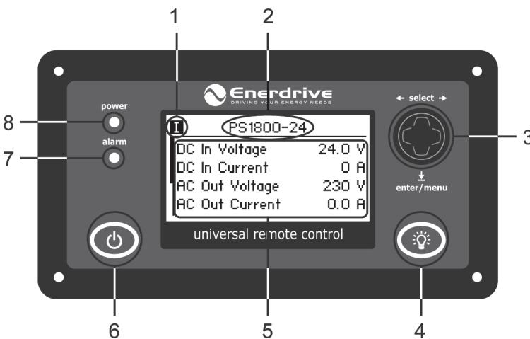
1. ePRO device mode indicator. With an inverter connected, symbol I indicates inverter on in normal mode. Symbol II indicates inverter on in ASB mode. With a charger connected, symbol I indicates charger on in normal mode. Symbol II indicates charger on in forced float mode. With a combi connected, symbol I indicates combi on in normal mode. Symbol II indicates combi on in charger only mode.
