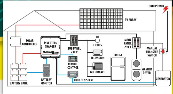
For reliable power, regardless of your application, the MagnaSine Inverter / Chargers, interconnecting system equipment and accessories are a solid base for back-up, or on-board power. Above are simple examples of how the MagnaSine system can fit into your application.
