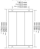
MOUNTING SCREW SPACING LENGTH \*(Hole diameter = 5.5 mm)
