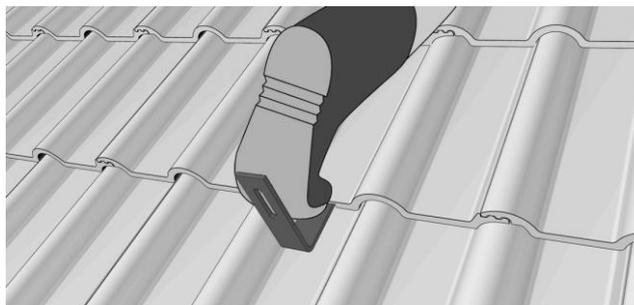
6. Variation for installation on plain tile roofs with plain tile roof cladding, a recess must be cut into the tiles around the position of the roof hook.
