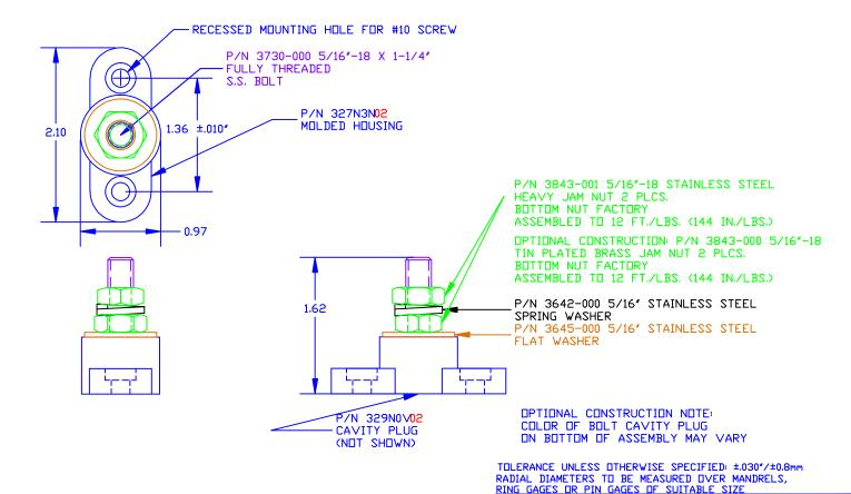
BASE MATERIAL: BASE MATERIAL U.L. RATING: DIELECTRIC STRENGTH VOLTAGE RATING: CURRENT RATING: TEMP, RISE AT LOAD:
