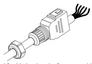
**Step 5** Connect the AC cable head to the European cold terminal by appropriate torque.
