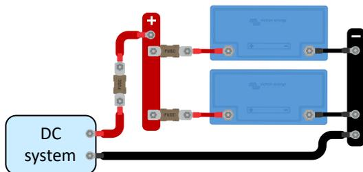
*Multiple batteries in parallel*
