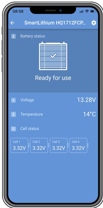
The battery is equipped with Bluetooth and uses this to communicate with the VictronConnect app. The VictronConnect app is used for reading out battery information, for making or changing battery settings, receiving alarms and to update firmware. VictronConnect also contains a demo modus.
