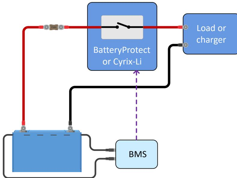
*The BMS controls the BatteryProtect or Cyrix-Li, which in turn disconnects the load or charger from the battery*
