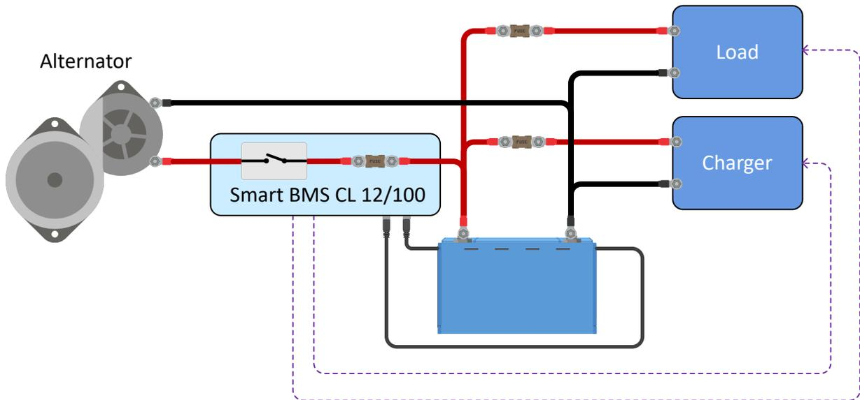
The Smart BMS CL 12/100 will turn loads and chargers off via "load disconnect" and "charge disconnect". It also controls and limits the alternator.
