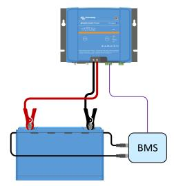
Initial charge with using a BMS
