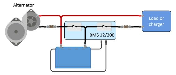
The BMS 12/200 disconnect loads and chargers. It also controls and current limits the alternator.
