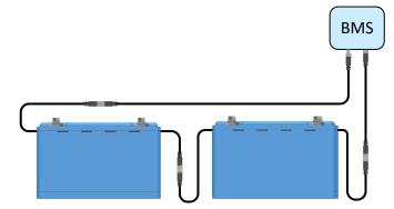
Multiple battery BMS connection with extension cables
