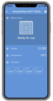
The battery is equipped with Bluetooth and uses this to communicate with the VictronConnect app. The VictronConnect app is used for reading out battery information, for making or changing battery settings, receiving alarms and to update firmware. VictronConnect also contains a demo modus.
