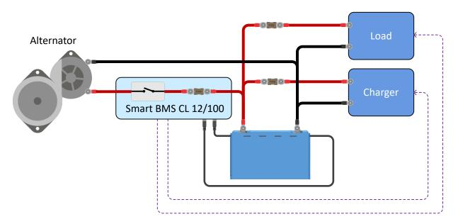
The Smart BMS CL 12/100 will turn loads and chargers off via "load disconnect" and "charge disconnect". It also controls and limits the alternator.
