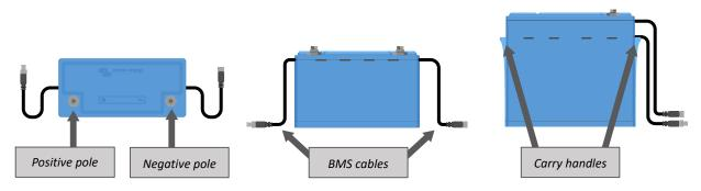
Top view battery showing battery terminals - Side view two different battery models showing BMS cables
