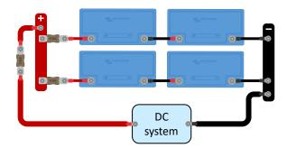
Multiple batteries in series/parallel
