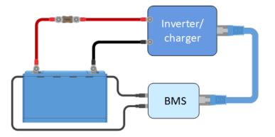
The BMS controls an inverter/charger directly via the VE.Bus
