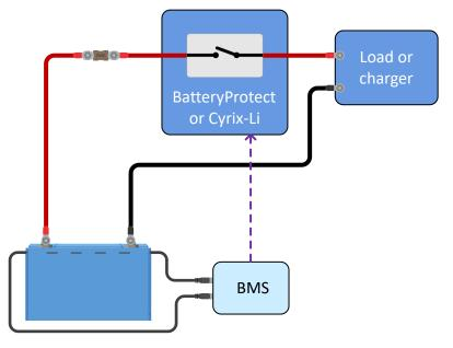
The BMS controls the BatteryProtect or Cyrix-Li, which in turn disconnects the load or charger from the battery
