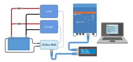
The VE.Bus BMS will turn loads and chargers off via "load disconnect", and "charge disconnect" and controls the inverter/charger
