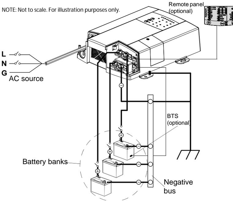
Figure 2-1 Typical Three-Battery Installation
