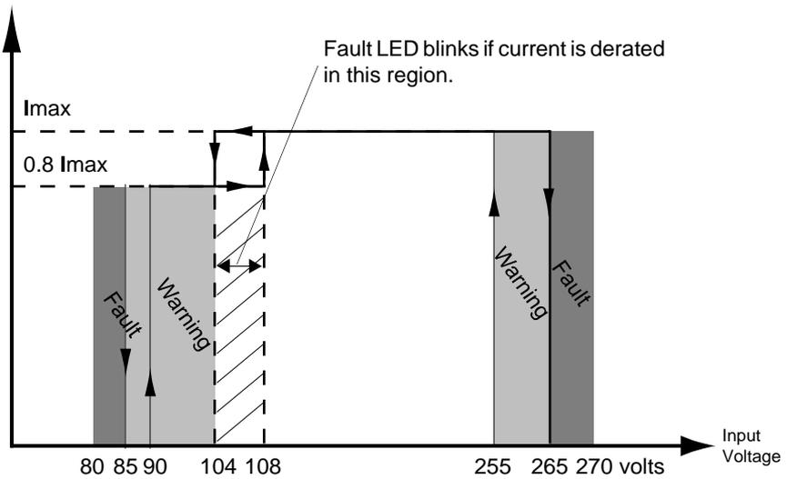
Figure 1-5 Input Voltage Operating and De-rating Curve
