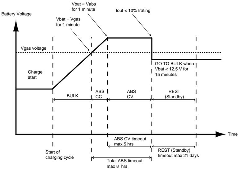
Figure 2-3 Two-Stage Charging Process
