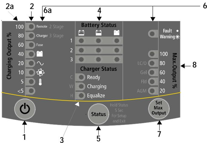
Figure 1-7 Truecharge™ 2 Battery Charger Remote Panel (optional)
