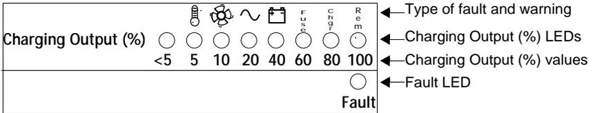
Figure 1-4 Charging Output (%) and Fault LEDs
