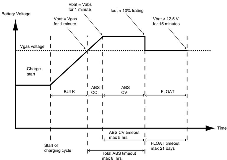
Figure 2-2 Three-Stage Charging Process
