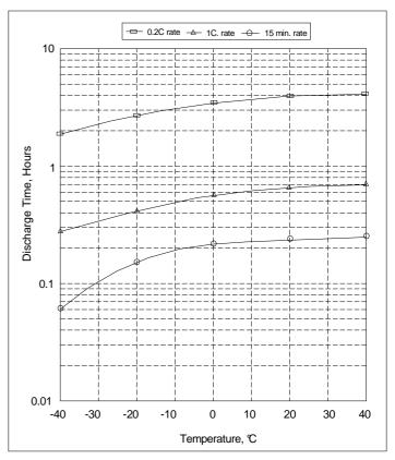
Figure 3: capacity Vs. Ambient Temperature
