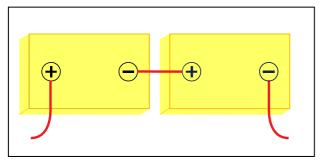
Example: Two HC110, 12V Batteries Rated at 110 AH Connected in Series
