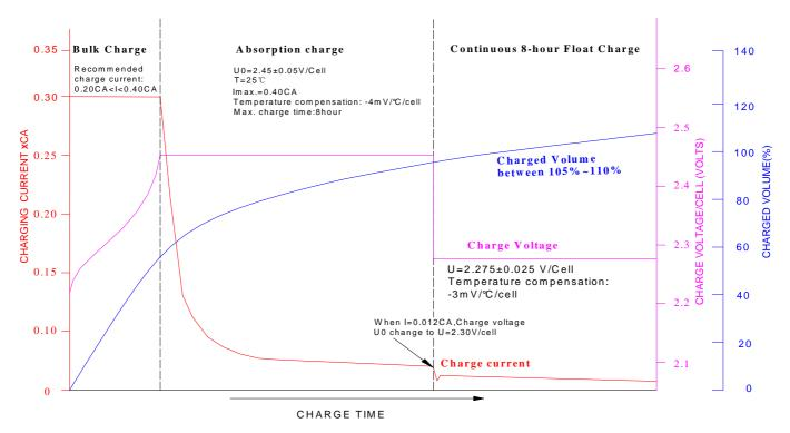
figure 5: Charging characteristics of a two constant voltage charger
