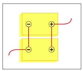
Example: Two HC110, 12V Batteries Rated at 110AH Connected in parallel
