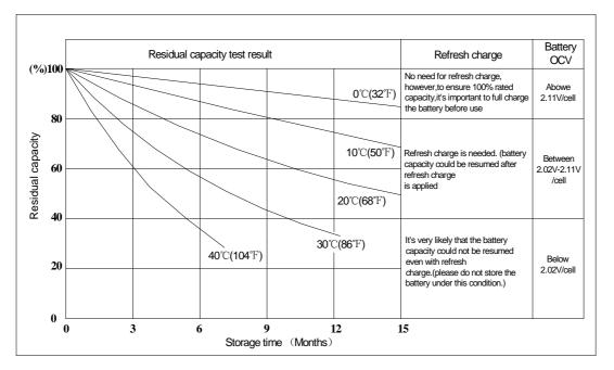
figure 1: Residual Capacity Vs. Storage time
