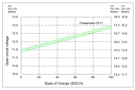
figure 2:Open Circuit Voltage Vs. State of Charge(SOC)
