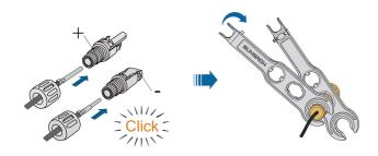
Step 4 Check for polarity correctness.
